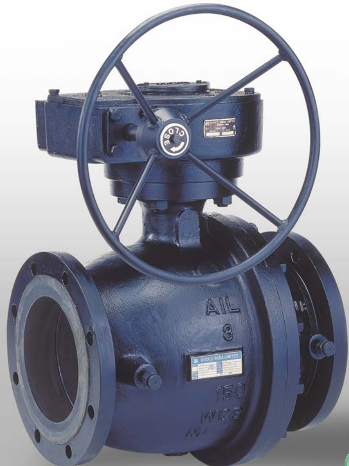
8" Full Bore Class 150 Bolted construction Gear-operated Metal seated Trunnion Mounted Ball Valve
